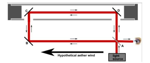
This apparatus was not spun or even moved, it was only aligned parallel (and then perpendicular) to the motion of the Earth. We are told that, given an ether, this experiment should have shown some difference between parallel and perpendicular, but it didn't. The result was negative.
