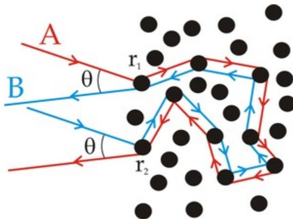
Propagation of two rays in a random medium. Since one can be obtained from the other by time inversion, they interfere coherently when the angle  $\theta$  goes to zero.
