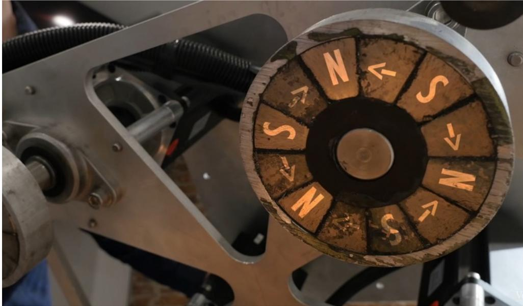
Above you can see an Halbach Array in one leg of the quadcopter and then they start to spin the array:
