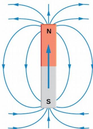
Magnetic field lines of a bar magnet
