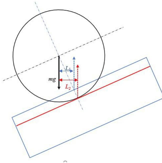
In essence, this means that, *ceteris paribus*, Peter's ball will *always* be *much slower* than Steven's ball in the straight line run, firstly because its *rotation* will be slower and secondly because the **first** effect reduces translation speed at any given speed of rotation.
