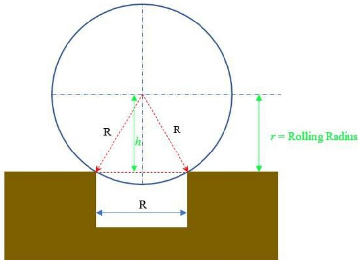
With a 3/4” diameter ball in a 3/8” wide slot, its two contact points and the ball centre form an equilateral triangle in a vertical plane, with each side of the triangle being 3/8” long. So, ball radius is  $R = 0.375$ ” and rolling radius is  $r$  is the vertical height ( $h$ ) of that equilateral triangle, i.e.
